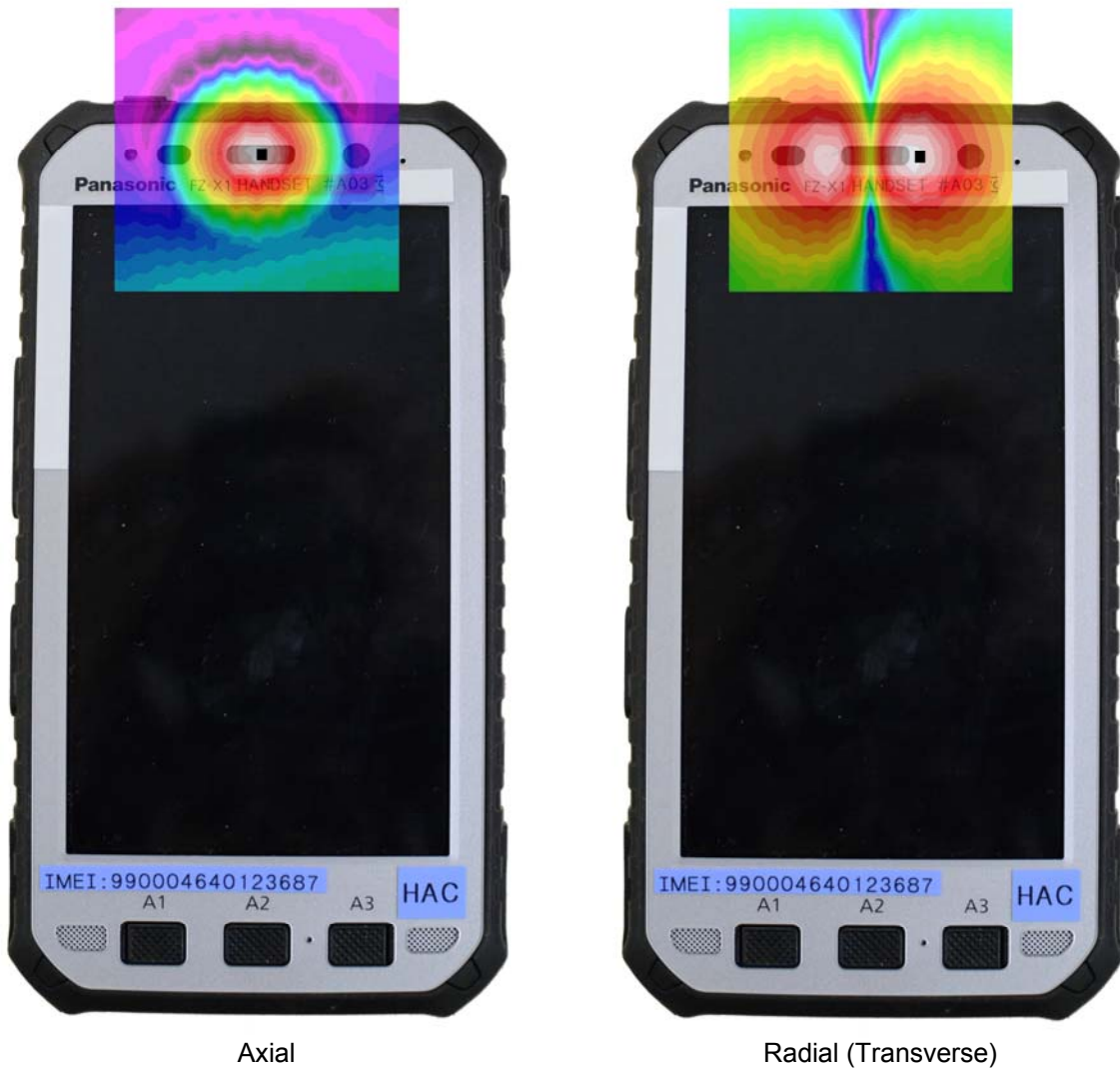
Axial Radial (Transverse) Figure 12-3 T-Coil Scan Overlay Magnetic Field Distributions
