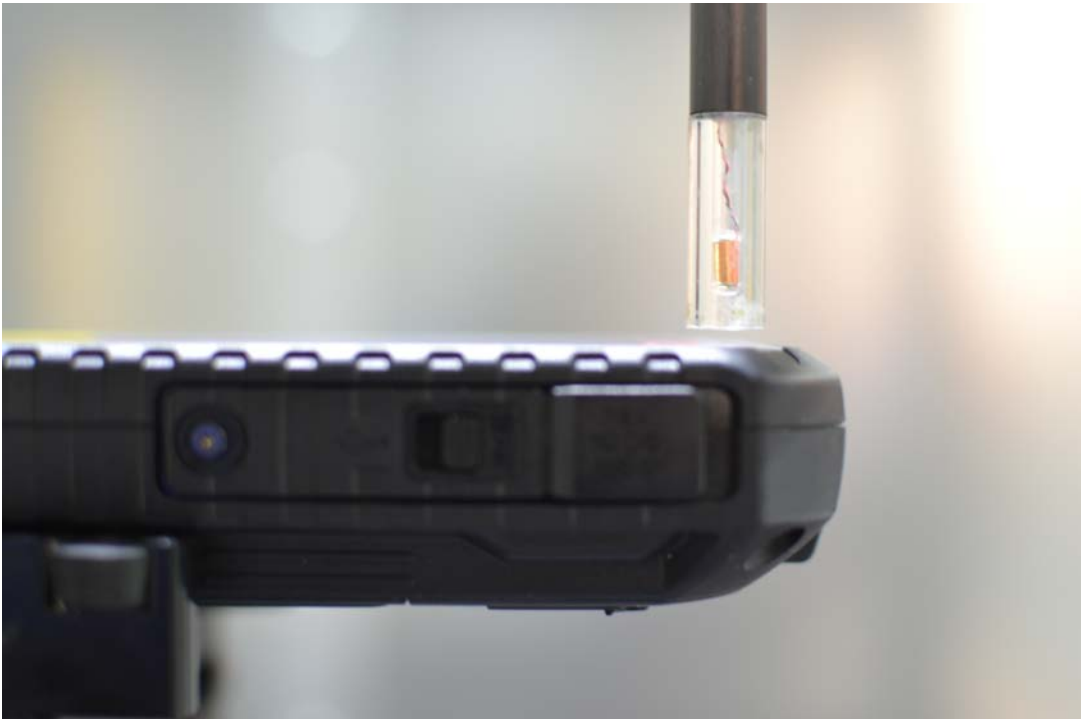
Figure 14-2 Test Setup for Wireless Device
