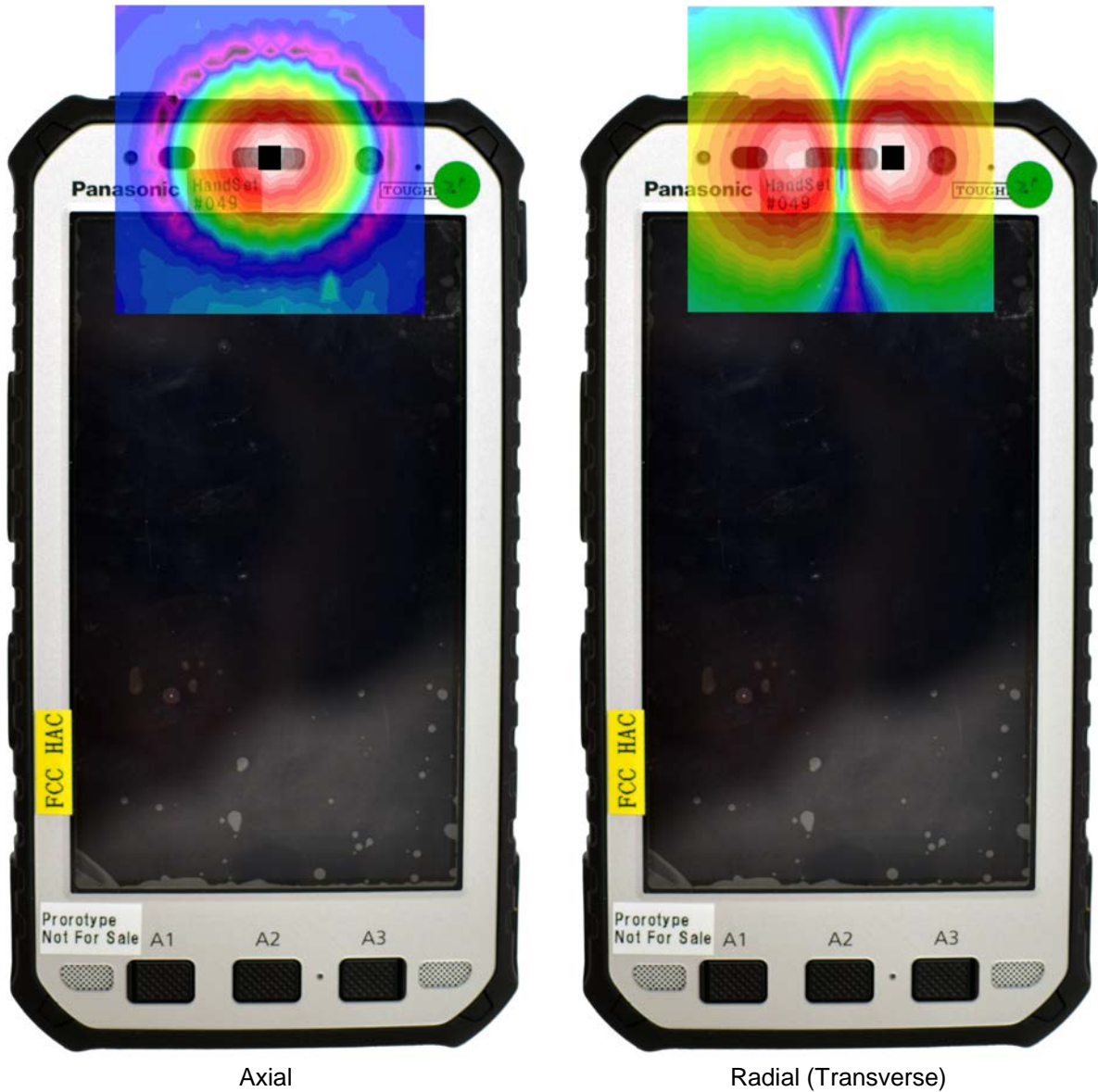
Figure 14-3 T-Coil Scan Overlay Magnetic Field Distributions
