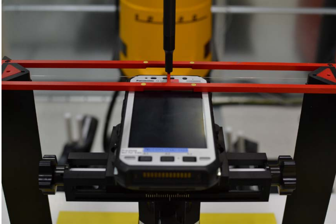
Figure 18-1 Ear Reference Point HAC Phantom Alignment
