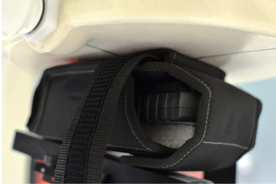
SAR Test Setup Photo 9: Back Side at 0.0 cm with Body Holster Accessory
