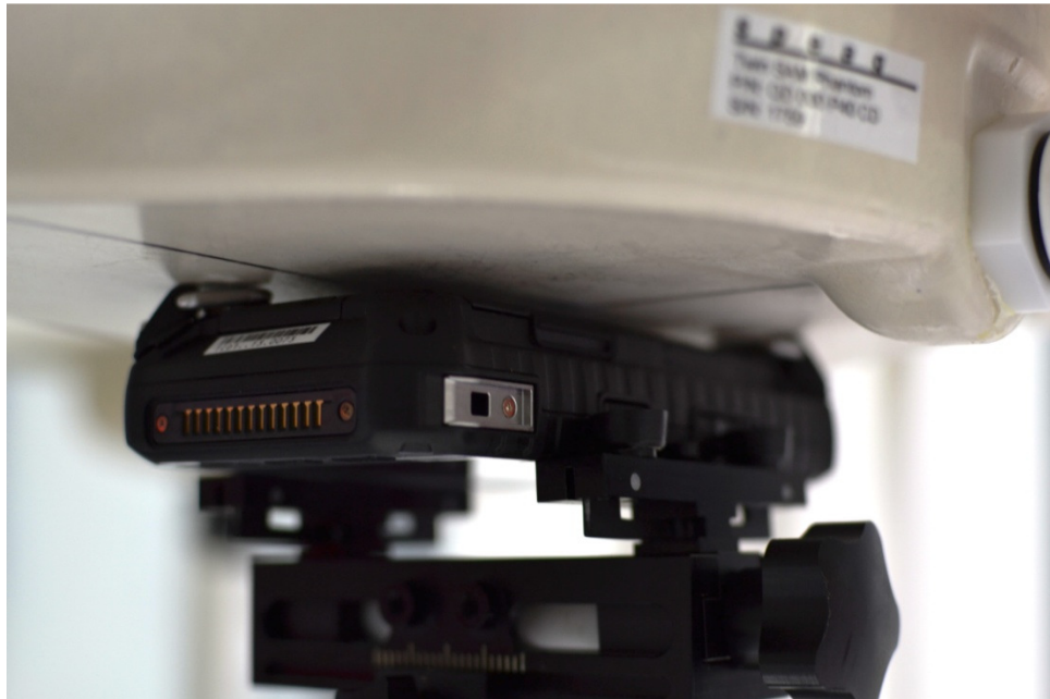
SAR Test Setup Photo 8 Back Side at 0.0 cm with Hand Strap Accessories (Top-Left)
