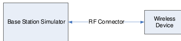
Figure 9-1 Power Measurement Setup
