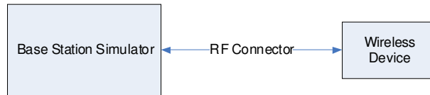
Figure 9-3 Power Measurement Setup
