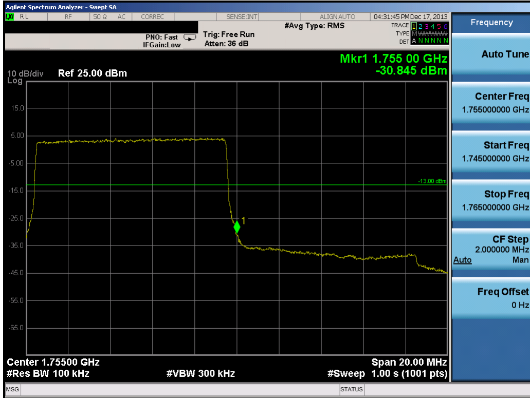
Plot 9-22. Upper Band Edge Plot (10.0MHz QPSK – RB Size 50)
