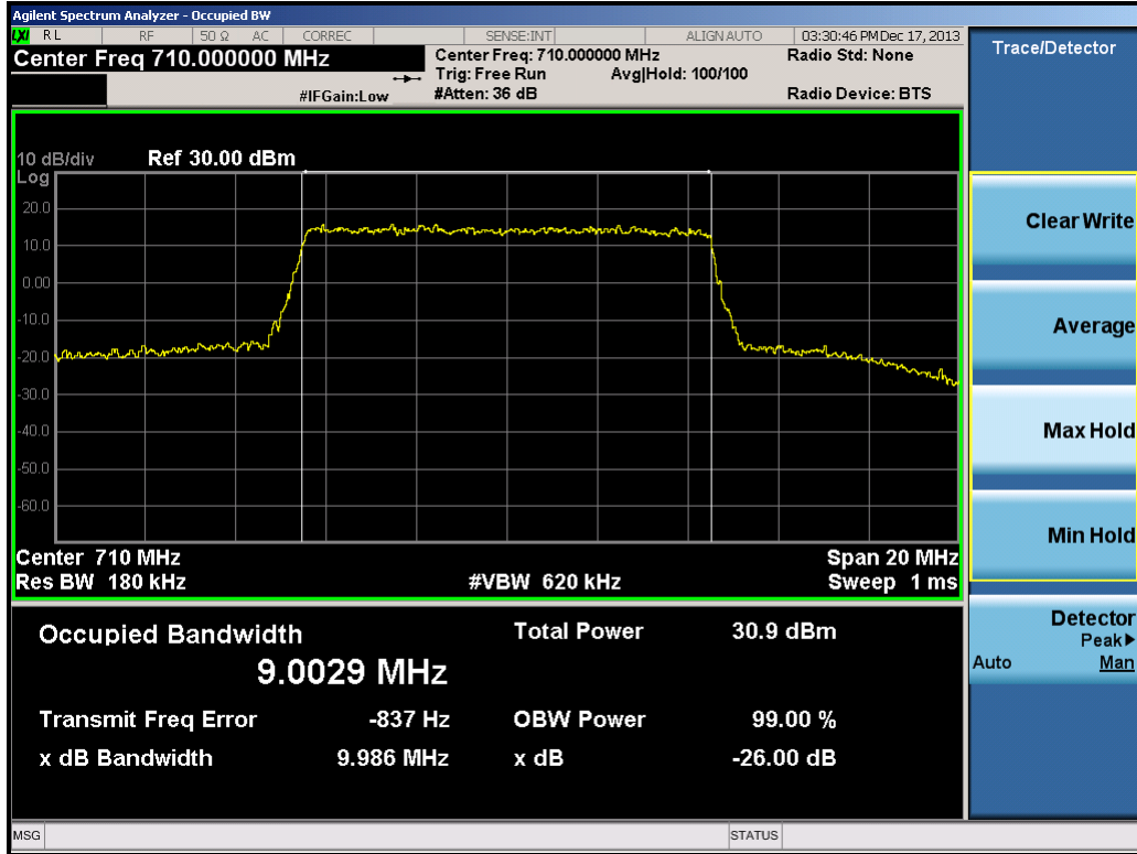
Plot 7-12. Occupied Bandwidth Plot (10.0MHz QPSK – RB Size 50)
