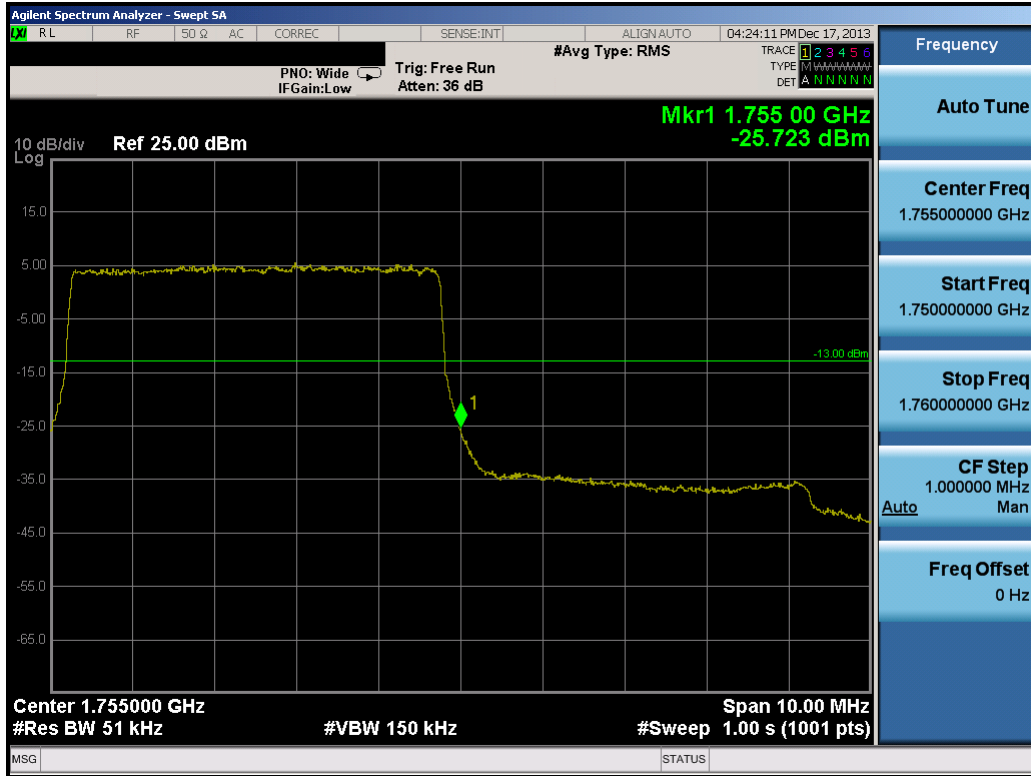
Plot 9-10. Upper Band Edge Plot (5.0MHz QPSK – RB Size 25)
