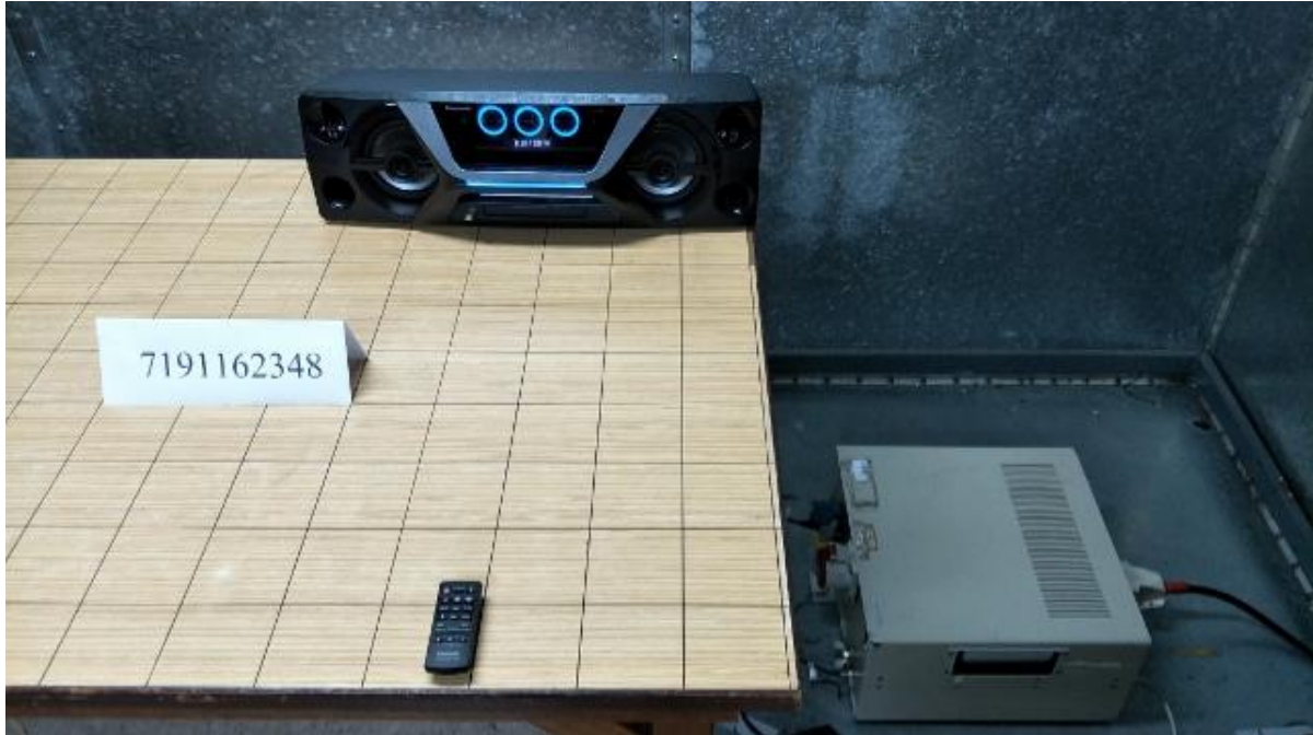
Conducted Emissions Test Setup (Front View)
