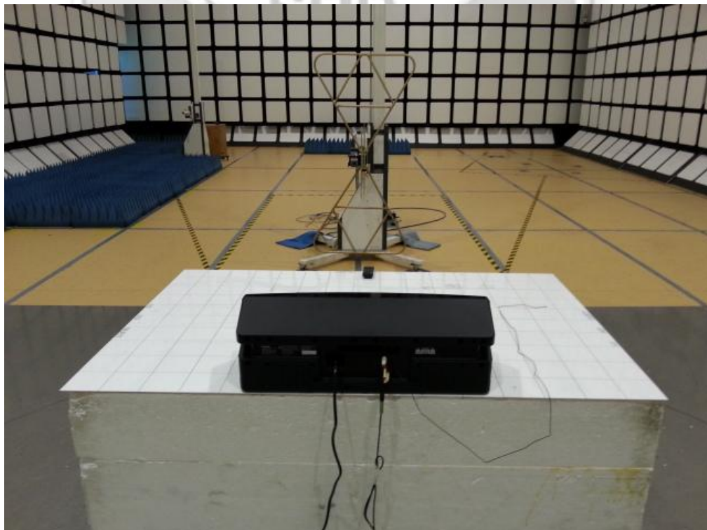
Radiated Emissions Test Setup (Rear View)
