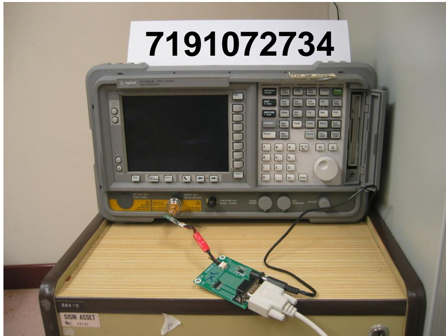
Average Frequency Dwell Time Test Setup
