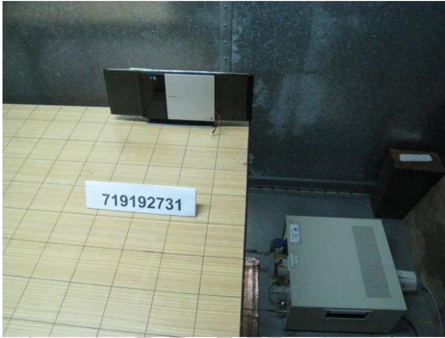
Conducted Emissions Test Setup (Front View)
