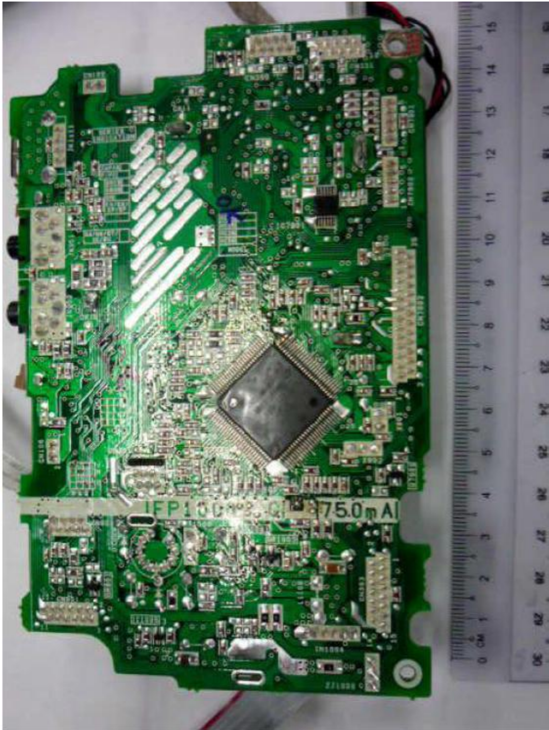
Main-Board PCB Trace Side
