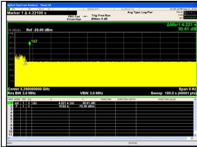
Radar at beginning of CAC – VHT80 – 5290MHz
