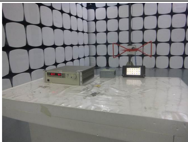
Radiated Spurious Emissions Test Setup Below 1GHz
