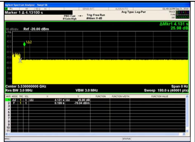
Radar at beginning of CAC – VHT80 – 5530MHz
