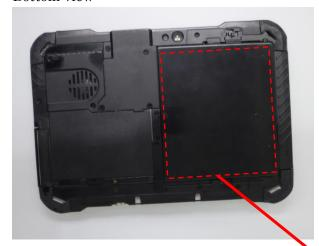
WLAN FCC ID and ISED certification number are to be printed on the nameplate.
