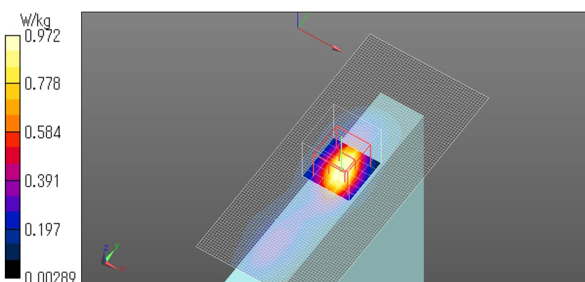
B.4 Plot No. W4.1 / Full/WCDMA B4 ch1312 1712.4MHz RMC,12.2 kbps Rear tilt Edge4 9mm
