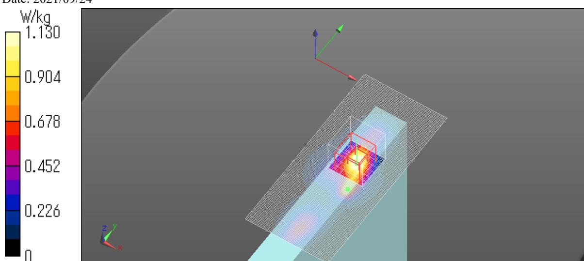
B.36 Plot No.ULCA41-1 / LTE Full 5 B41(SCC1 40422) ch40620 2593MHz QPSK NA Rear tilt edge1 0mm 20MHz RBn1 RBp0
