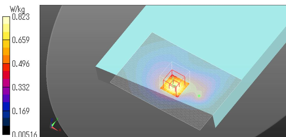
B.25 Plot No. L25.2 / Red/LTE B25 ch26140 1860MHz QPSK Edge4 0mm 20MHz RBn100 RBp0
