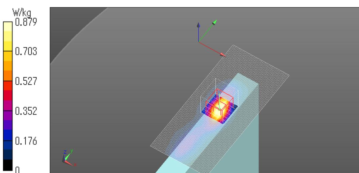
B.46 Plot No. N5.1 / Full /NR Bn5 ch167300 836.5MHz BPSK DFTsOFDM Rear tilt Edge4 9mm 20MHz RBn50 RBp28
