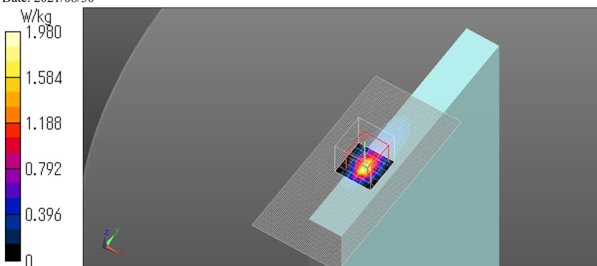
B.50 Plot No. N66.1 / Full/NR Bn66 ch344000 1720MHz BPSK DFTsOFDM Rear tilt Edge4 9mm 20MHz RBn50 RBp28
