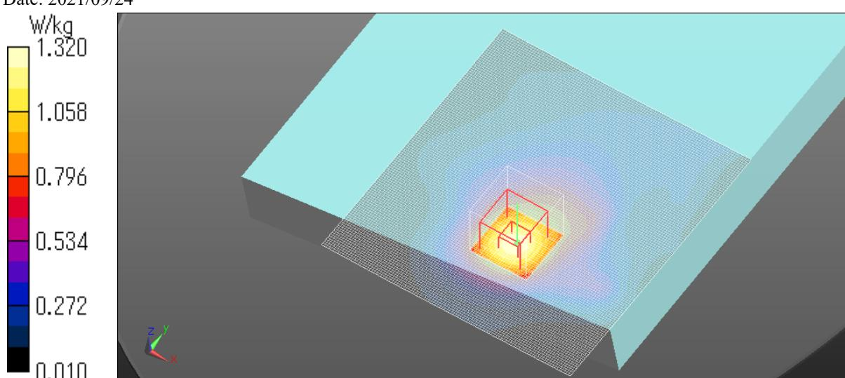
B.35 Plot No.ULCA7-2 / LTE Red 5 B7(SCC 21298) ch21100 2535MHz QPSK DFTsOFDM Edge4 0mm 20MHz RBn1 RBp99
