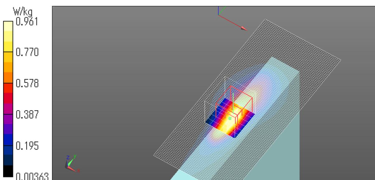
B.24 Plot No. L25.1 / Full /LTE B25 ch26140 1860MHz QPSK Rear tilt Edge1 20MHz RBn1 RBp0
