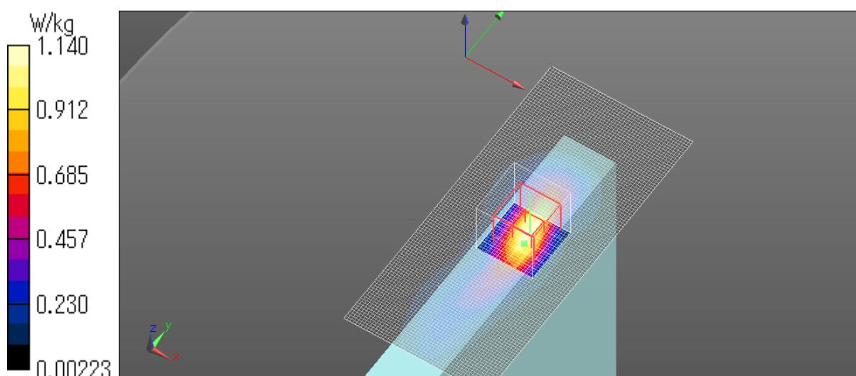
B.42 Plot No. L71.1 / Full/LTE B71 ch133297 680.5MHz QPSK Rear tilt Edge4 9mm 20MHz RBn1 RBp99
