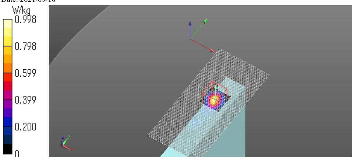
B.40 Plot No. L66.1 / Full /LTE B66 ch132072 1720MHz QPSK Rear tilt Edge4 9mm 20MHz RBn1 RBp99
