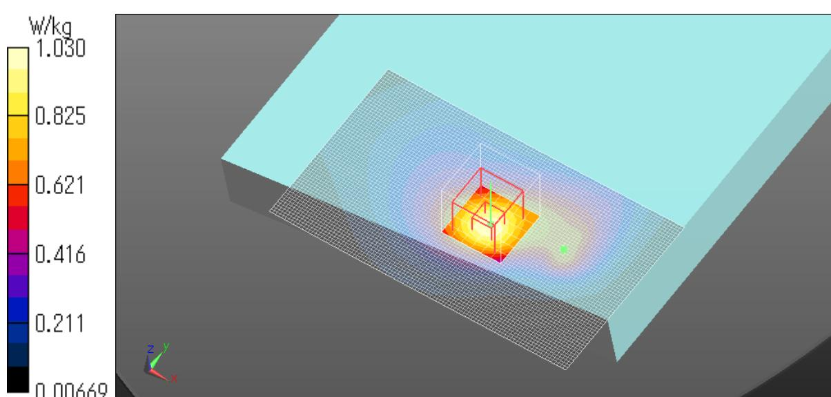
B.3 Plot No. W2.2 / Red/WCDMA B2 ch9538 1907.6MHz RMC,12.2 kbps Edge4 0mm
