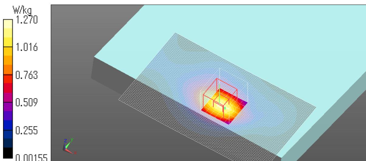
B.41 Plot No. L66.2 / Red/LTE B66 ch132572 1770MHz QPSK Edge4 0mm 20MHz RBn100 RBp0
