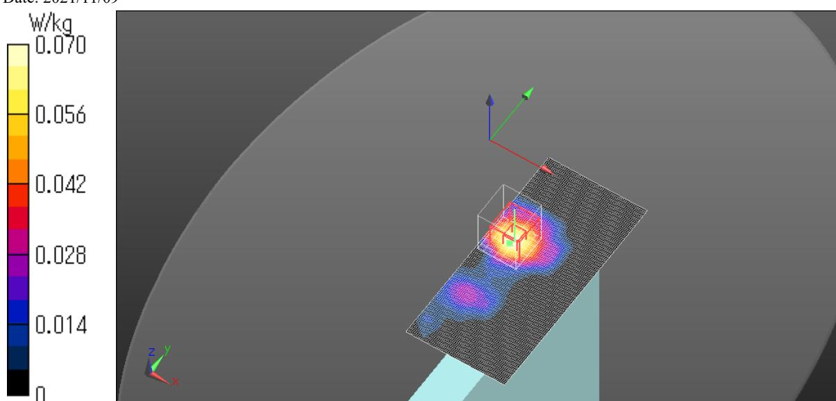
B.39 Plot No.ULCA48-2 / LTE Red 5 B48(SCC1 55340) ch55340 3560MHz QPSK DFTsOFDM Edge4 0mm 20MHz RBn50 RBp49
