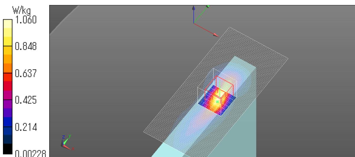
B.12 Plot No. L5.1 / Full/LTE B5 ch20525 836.5MHz QPSK Rear tilt Edge1 0mm 10MHz RBn1 RBp0
