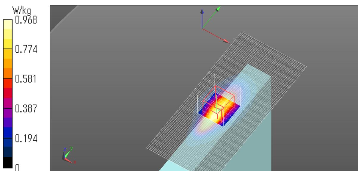
B.22 Plot No. L17.1 / Full/LTE B17 ch23790 710MHz QPSK Rear tilt Edge1 0mm 10MHz RBn1 RBp49
