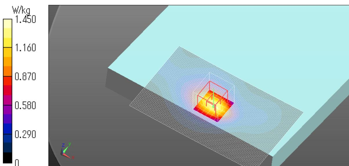
B.5 Plot No. W4.2 / Red/WCDMA B4 ch1413 1732.6MHz RMC,12.2 kbps Edge4 0mm
