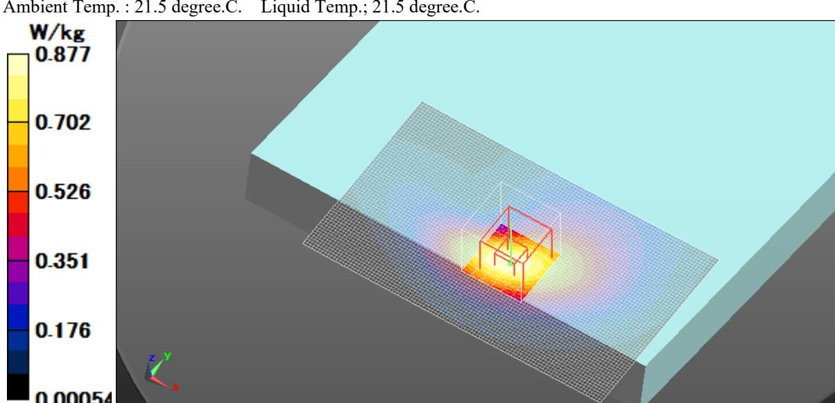
B.27 Plot No. L26.2 / Red/LTE B26 ch26865 831.5MHz QPSK Edge4 0mm 15MHz RBn75 RBp0
