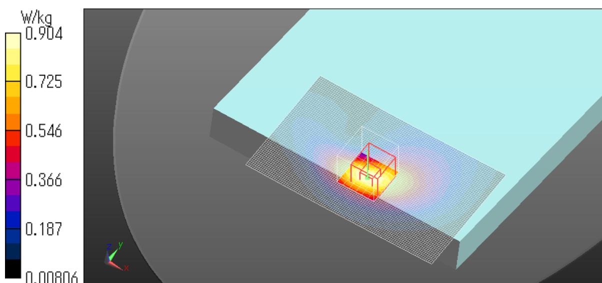
B.7 Plot No. W5.2 / Red/WCDMA B5 ch4233 846.6MHz RMC,12.2 kbps Edge4 0mm
