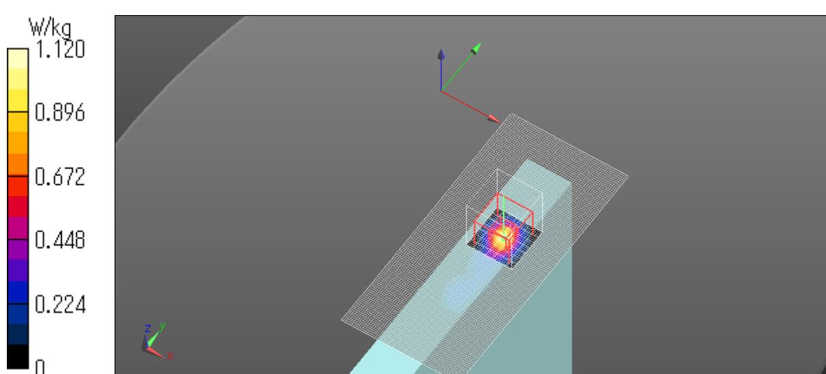
B.34 Plot No.ULCA7-1 / LTE Full 5 B7(SCC 20902) ch21100 2535MHz QPSK NA Rear tilt edge1 0mm 20MHz RBn1 RBp0
