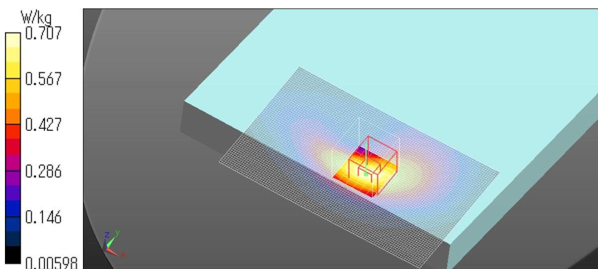
B.43 Plot No. L71.2 / Red/LTE B71 ch133297 680.5MHz QPSK Edge4 0mm 20MHz RBn1 RBp99
