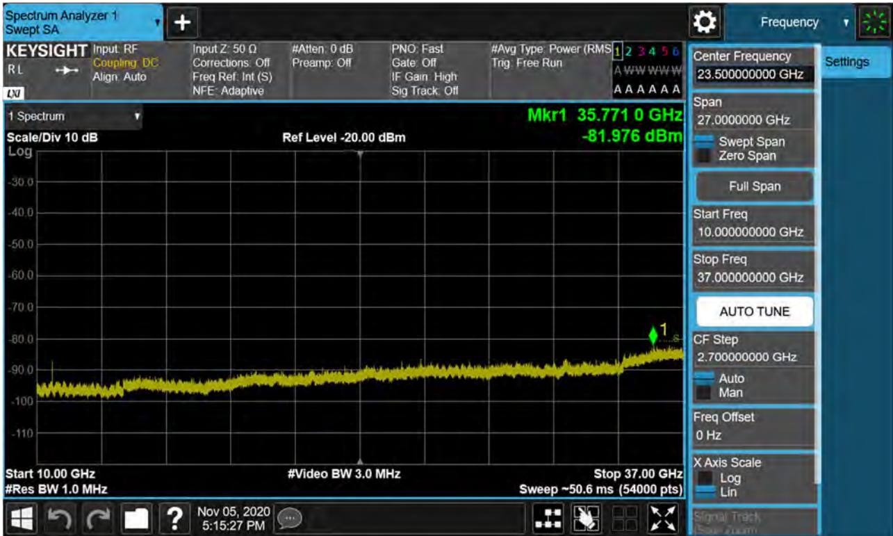
BAND 48. Conducted Spurious Plot 2 (10 MHz Ch. 55290 QPSK RB 1, Offset 0)
