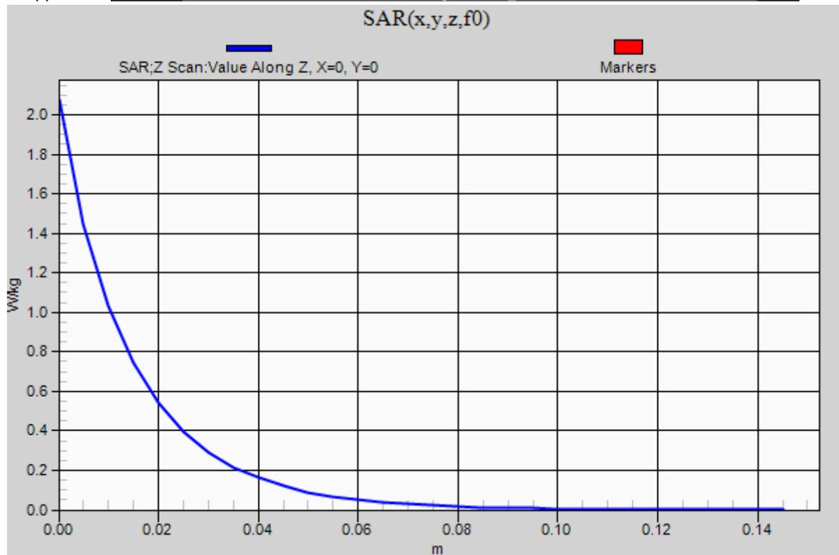
**20180425 Body 1750MHz System Check Power 250mW**
