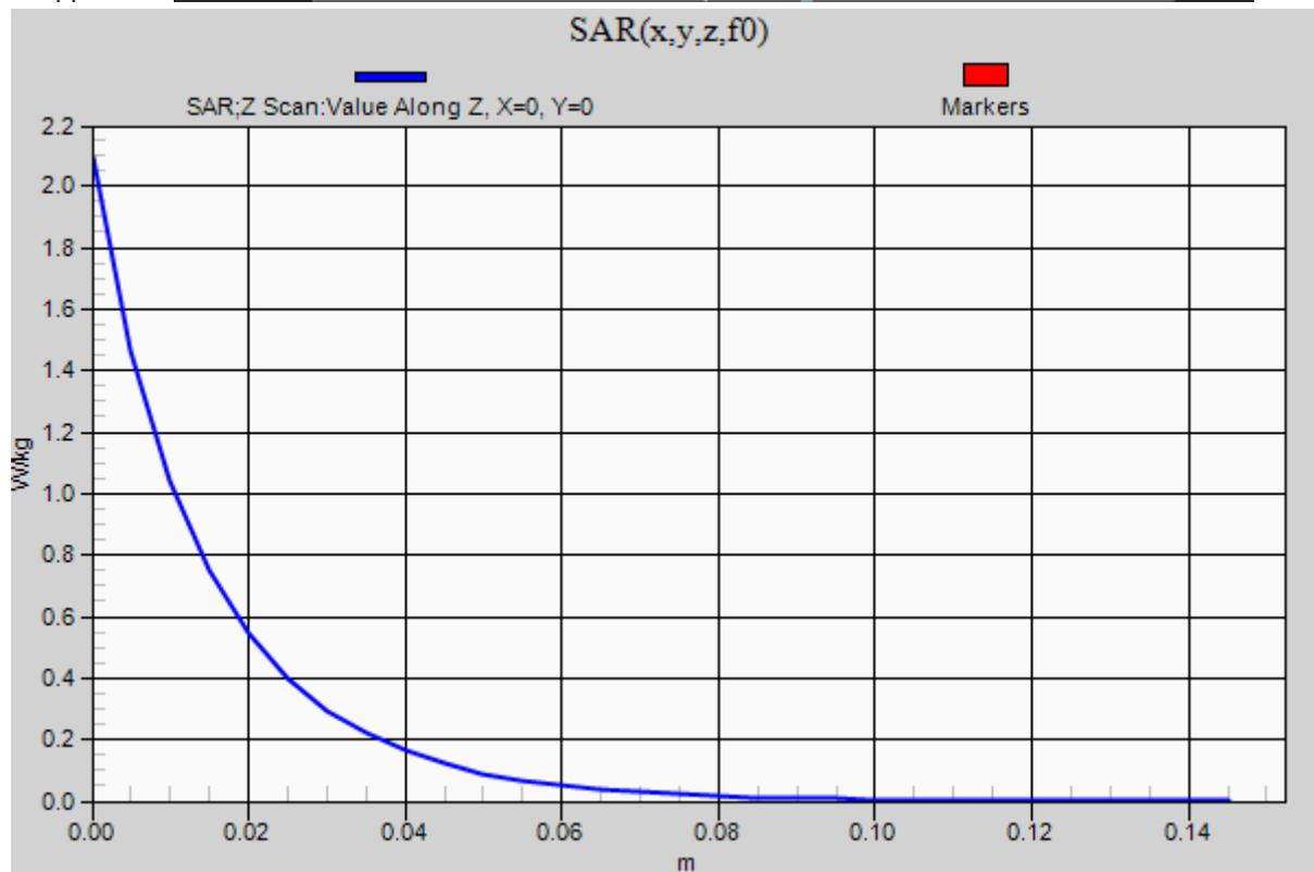
**20180424 Body 835MHz System Check Power 250mW**
