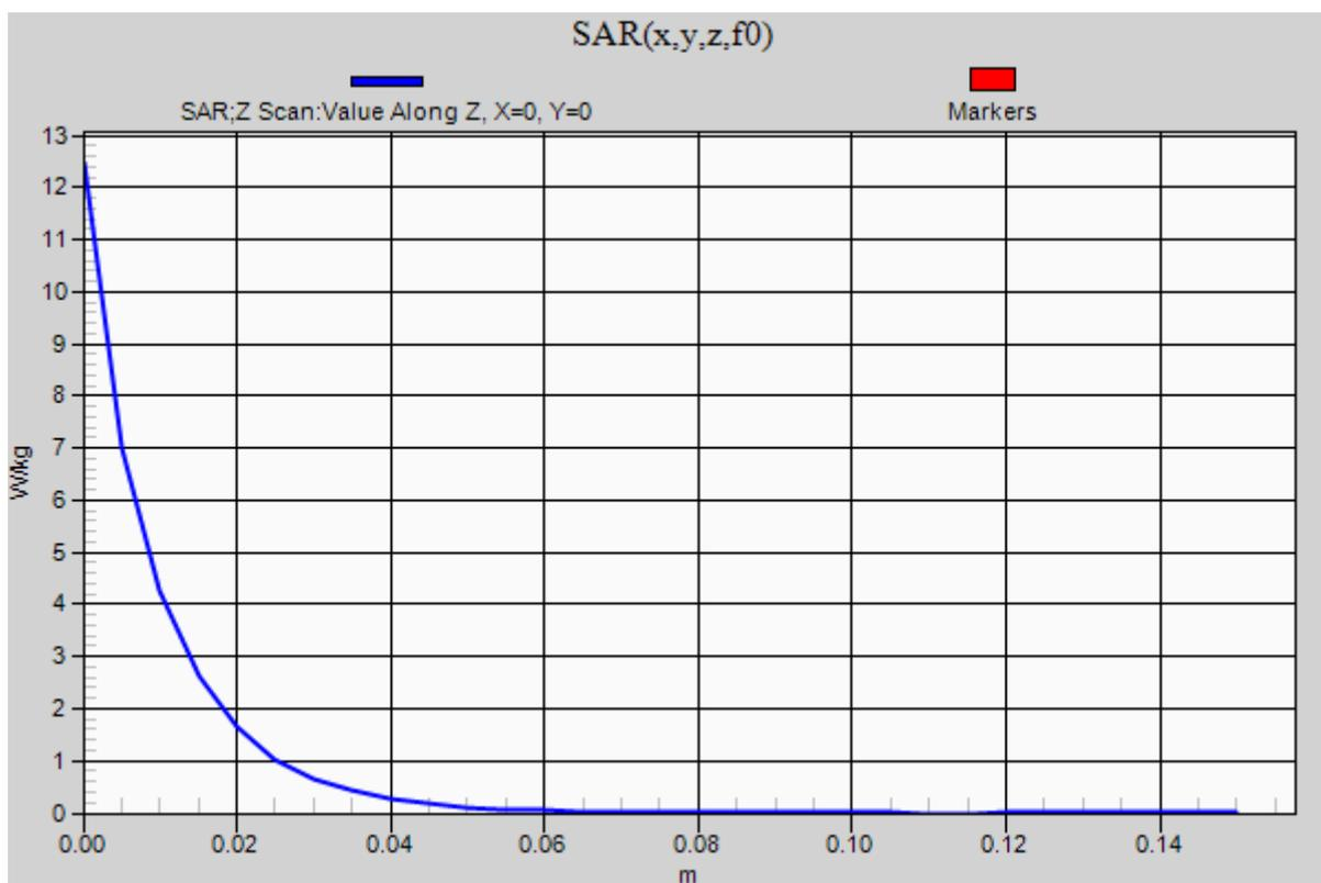
**20180425 Body 835MHz System Check Power 250mW**
