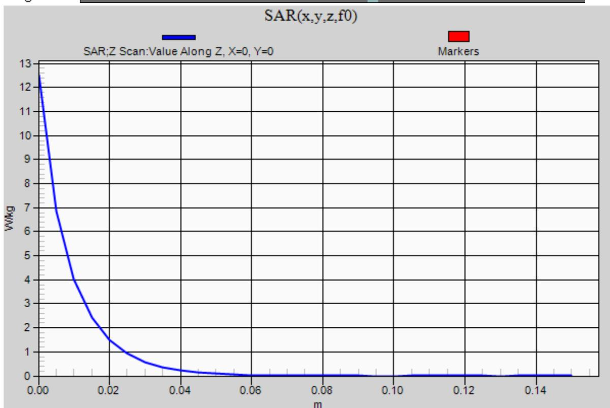
**20180423 Body 835MHz System Check Power 250mW**
