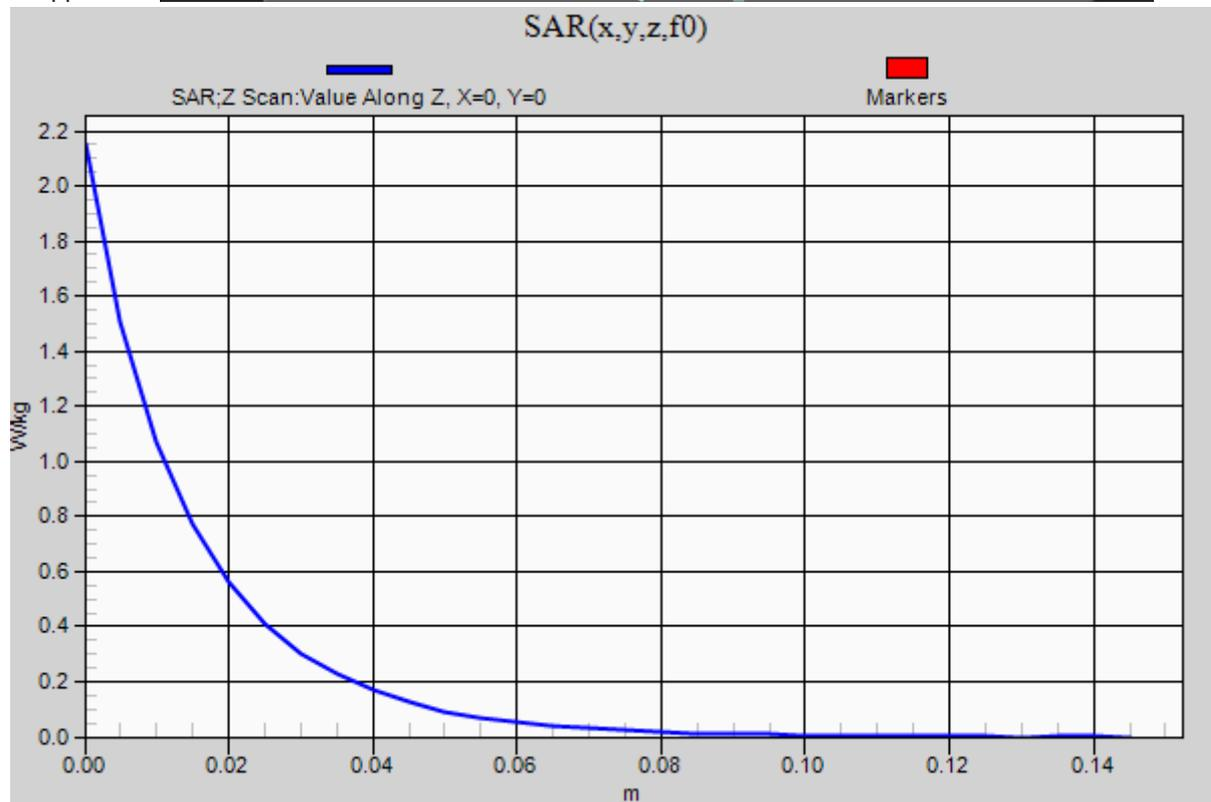
**20180424 Body 1750MHz System Check Power 250mW**
