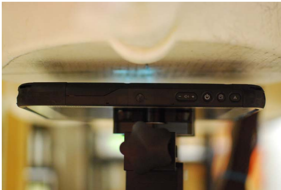
SAR Test Setup Photo 2: Back at 1.9 cm
