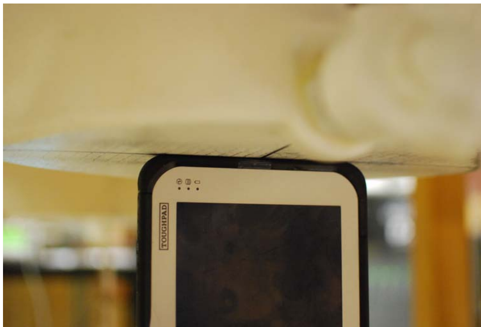
SAR Test Setup Photo 4: Right at 0.0 cm
