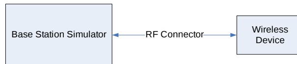
Figure 8-1 Power Measurement Setup
