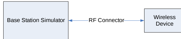
Figure 8-2 Power Measurement Setup
