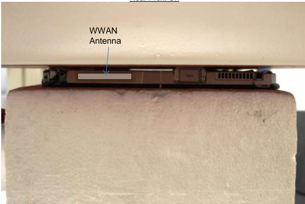
Edge 1 Prox. On, 0 mm Separation Distance
