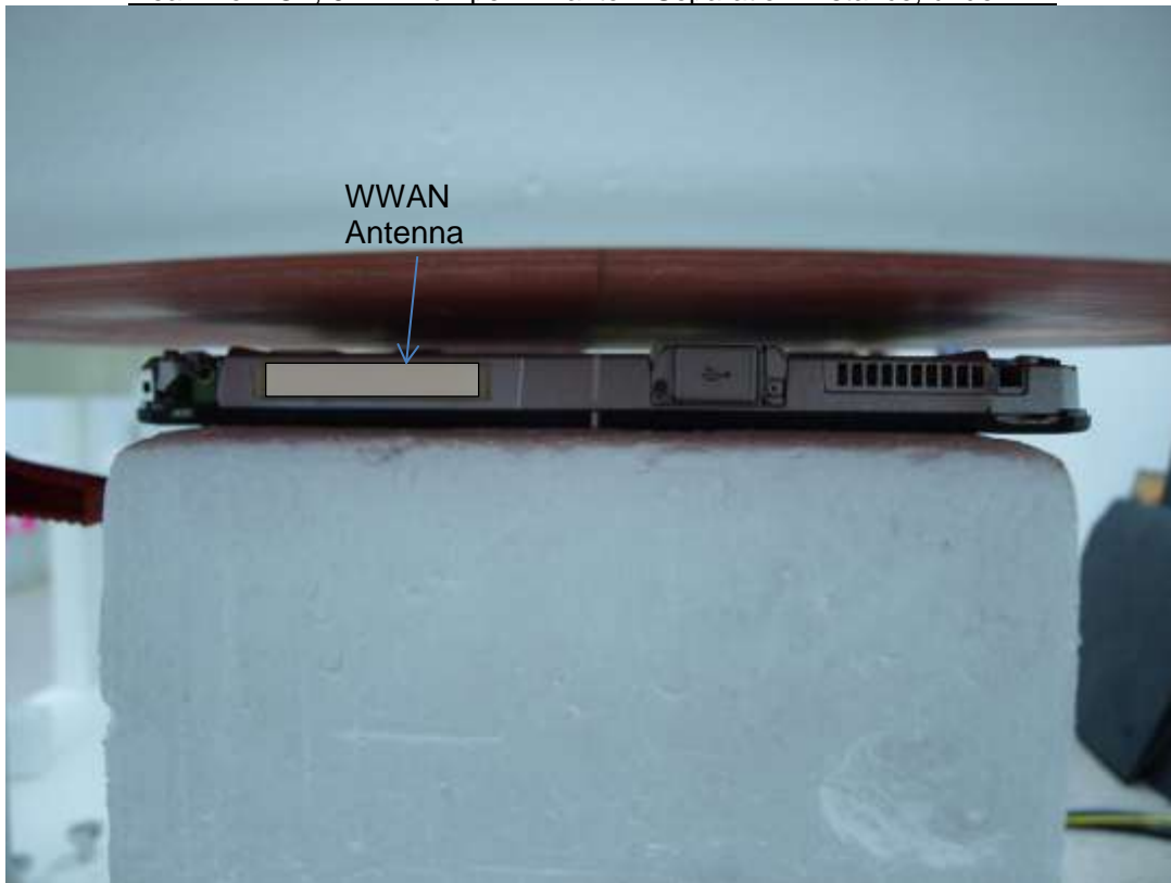
Edge 1 Prox. Off, 20 mm Separation Distance
