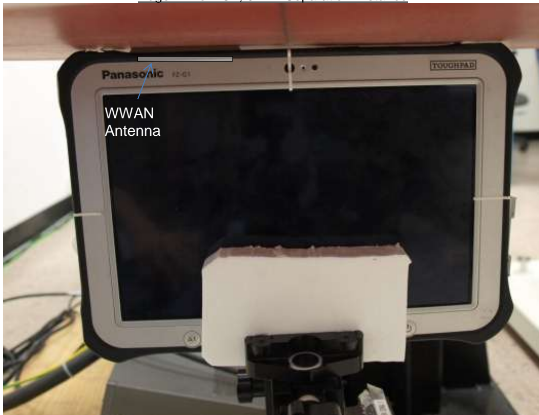
Edge 1 Prox. On, 0 mm Separation Distance
