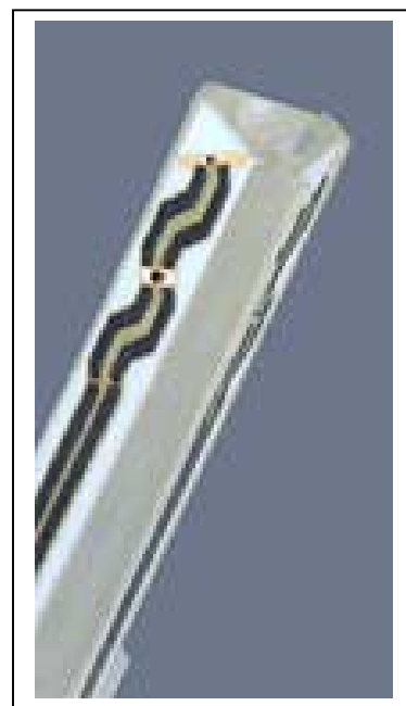
Figure. Inside view of ET3DV6 E-field Probe
