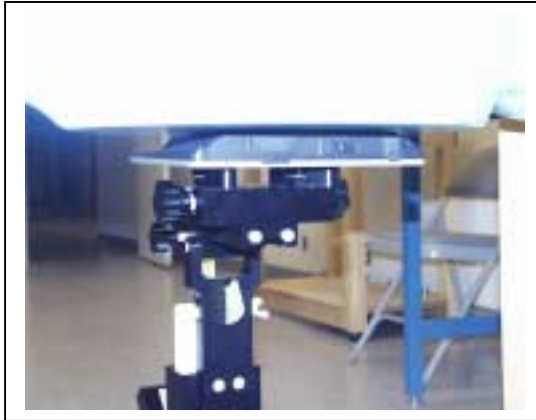
Figure. Abnormal test position for reference only (When EUT bottom side face the stomach)
