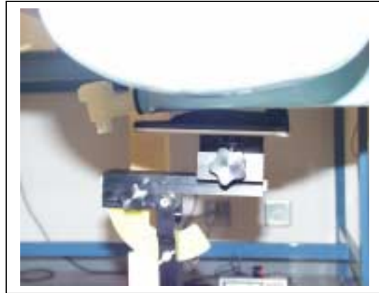
Figure. Abnormal test position for reference only (When EUT bottom side face the stomach)
