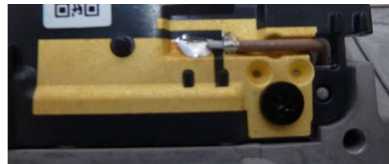
The close-up photo of the WLAN #2 /Bluetooth Antenna
