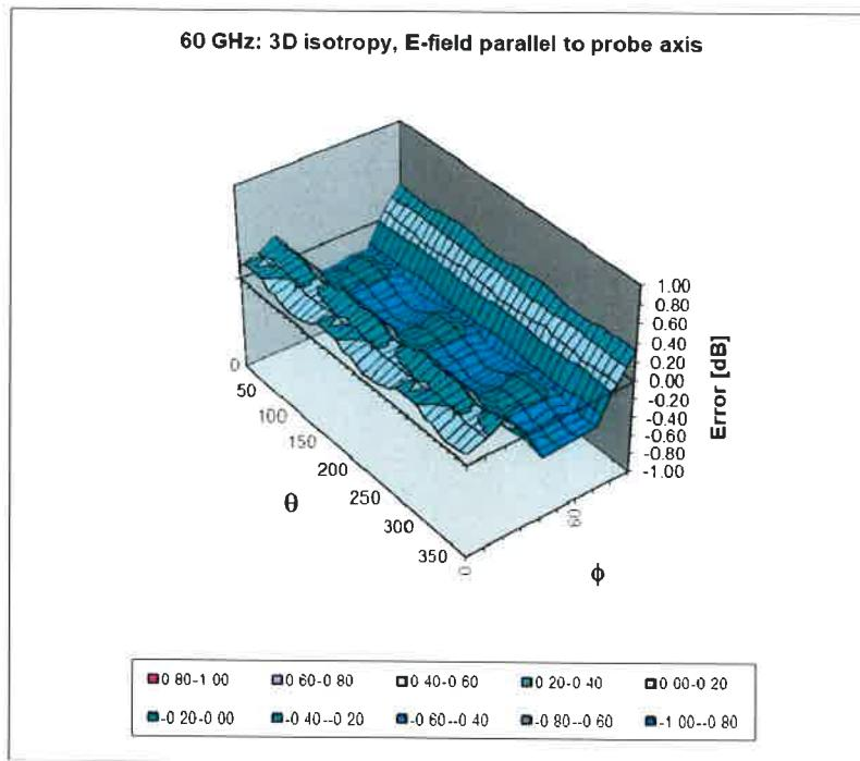
Probe isotropy for  $E_{\text{tot}}$ : probe rotated  $\phi = 0^\circ$  to  $360^\circ$ , tilted from field propagation direction  $\bar{k}$
