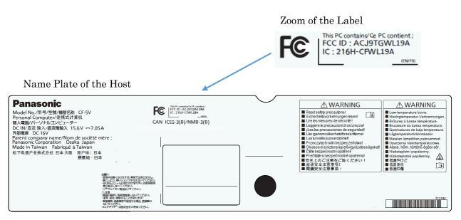
\*This label is printed on the Name Plate which is to be attached on the Host.
