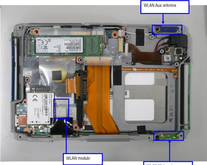
2-2) Enlarged view of WLAN module
