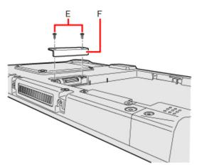
8. Insert the battery pack.( PReplacing the Battery Pack)
