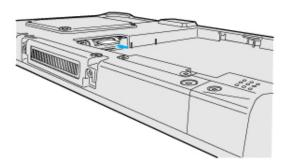
7. Close the SIM card slot cover(F), attach it and tighten the screw (E) firmly.
