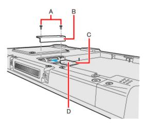
5. Insert the SIM card (C) into the SIM card slot with the contact side (D) facing downward and with the cut corner oriented as shown in the illustration.
