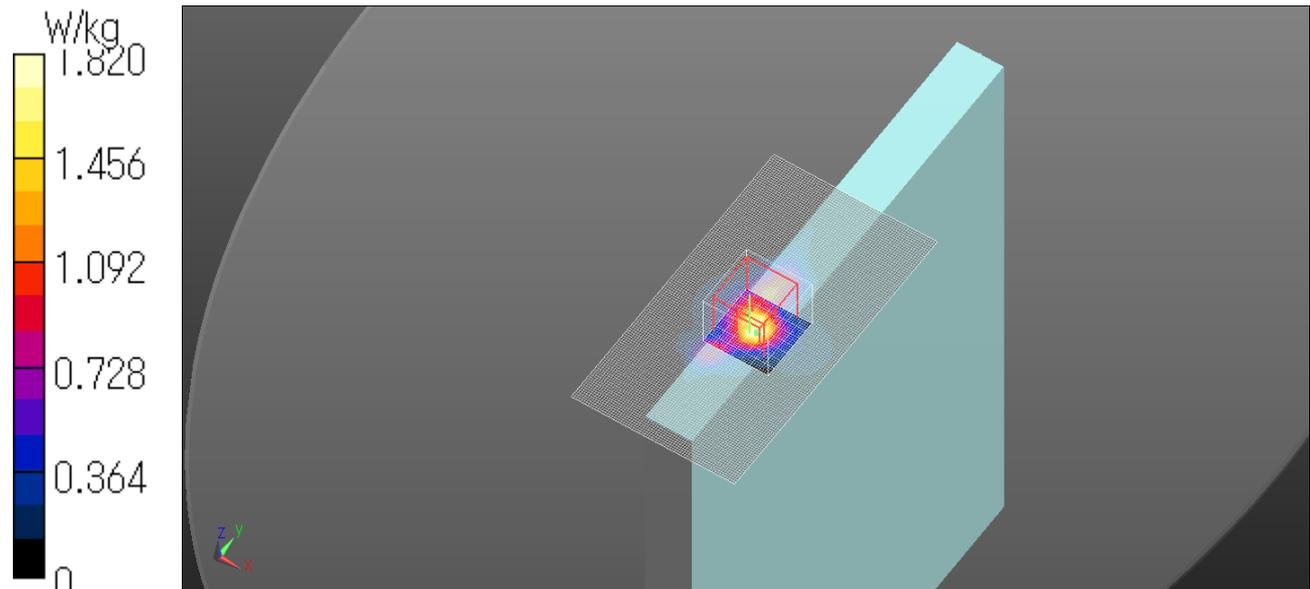
**WLAN 5.5G Main Ant Rear 11ac80 VHT0 0mm 5690MHz**
