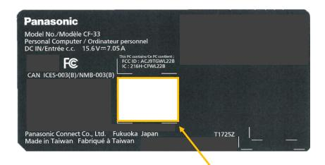
1.1 Label for RFID module on the host
