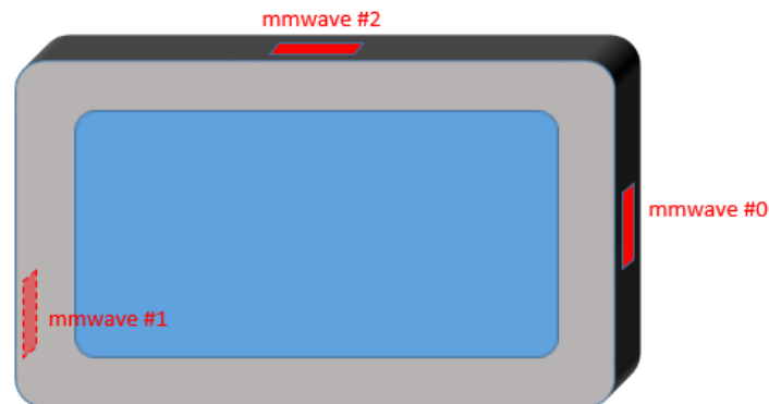
Figure 2. Simulation model which is mounted three mmWave antenna modules.
