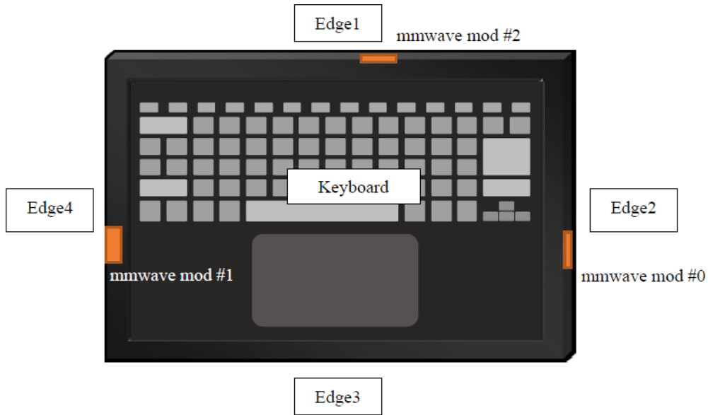
Figure 2. Simulation model which is mounted three mmWave antenna modules.
