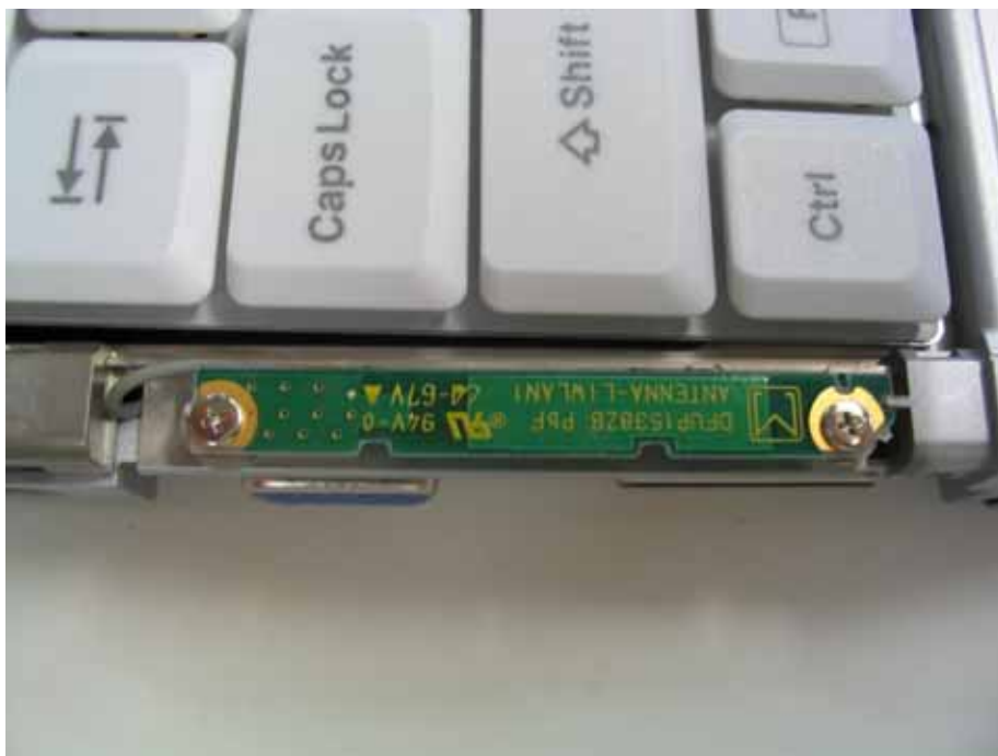
WLAN AUX TX/RX Antenna
