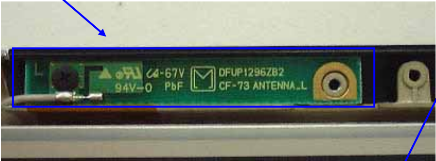
Aux TX/RX Antenna View
