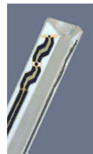
Figure 3.2 Probe Thick-Film Technique
