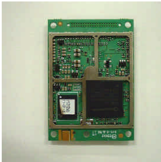
SB555 Module Interior Top View
