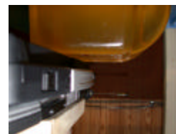
Figure A.2 Body SAR Test Setup -- Lap Position --
