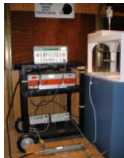
Figure A.0 Dipole Validation Test Setup
