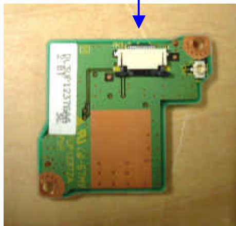
Bottom View of Bluetooth Module with Daughter Board
