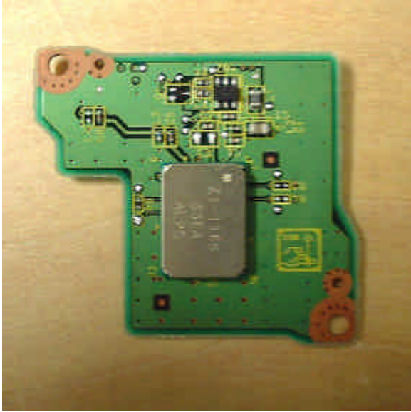
Top View of Bluetooth Module with Daughter-Board
