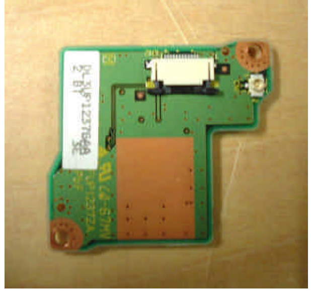
Bottom View of Bluetooth module with Daughter-Board
