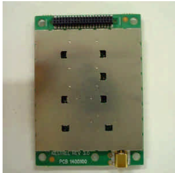
SB555 module Bottom View
