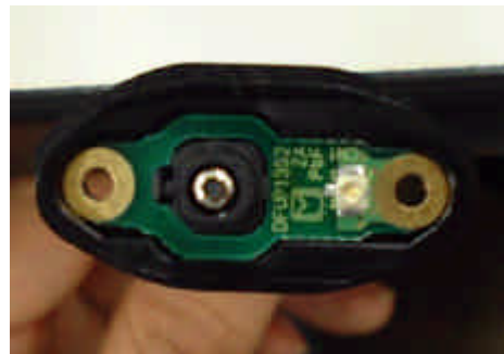
Whip Antenna I/F PCB
