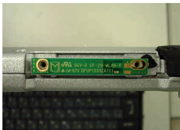
Send & Receive Antenna View
