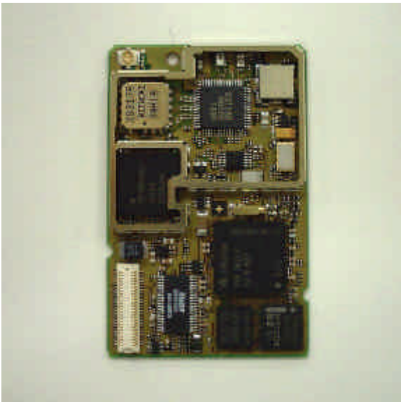
MC46 Module Interior View
