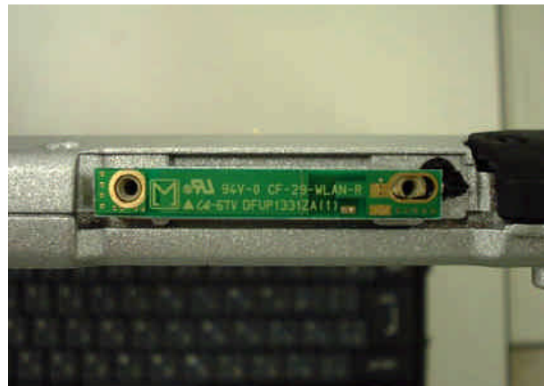
Send & Receive Antenna View
