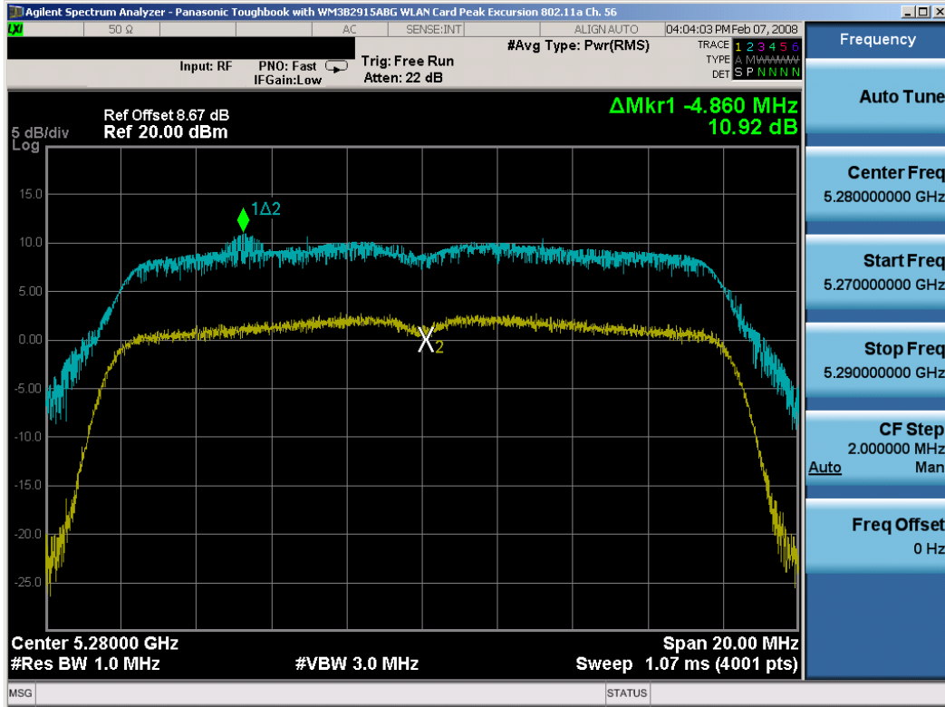
Plot 6-17. Excursion Ratio Plot (802.11a (UNII) – Ch. 56)
