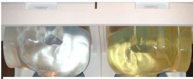
Figure 7.1 Left and Right SAM Phantom shells
