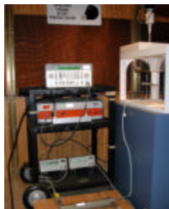
Figure A.0 Dipole Validation Test Setup
