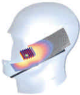
Figure 7.1 Sample SAR Area Scan
