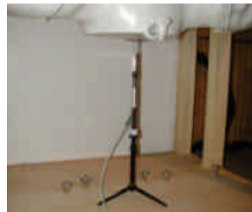
Figure 12.1 Dipole Validation Test Setup
