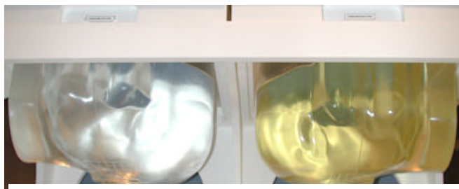
Figure 7.1 Left and Right SAM Phantom shells
