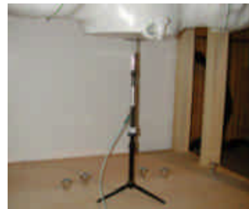
Figure 12.1 Dipole Validation Test Setup
