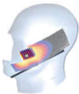
Figure 7.1 Sample SAR Area Scan
