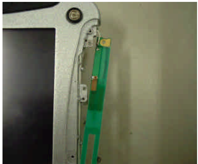
Antenna Magnified View
