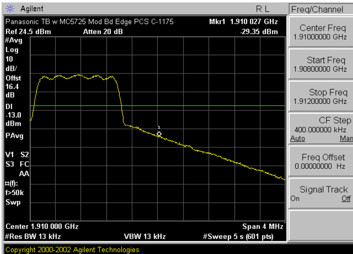
Plot A-21. Band Edge Plot (PCS CDMA Mode – Ch. 1175)
