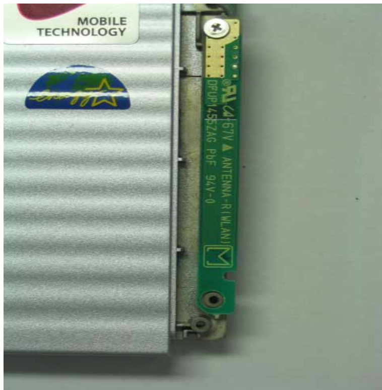
Main TX/RX Antenna magnified View
