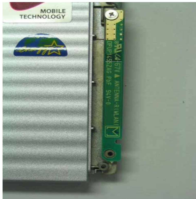
Main TX/RX Antenna magnified View
