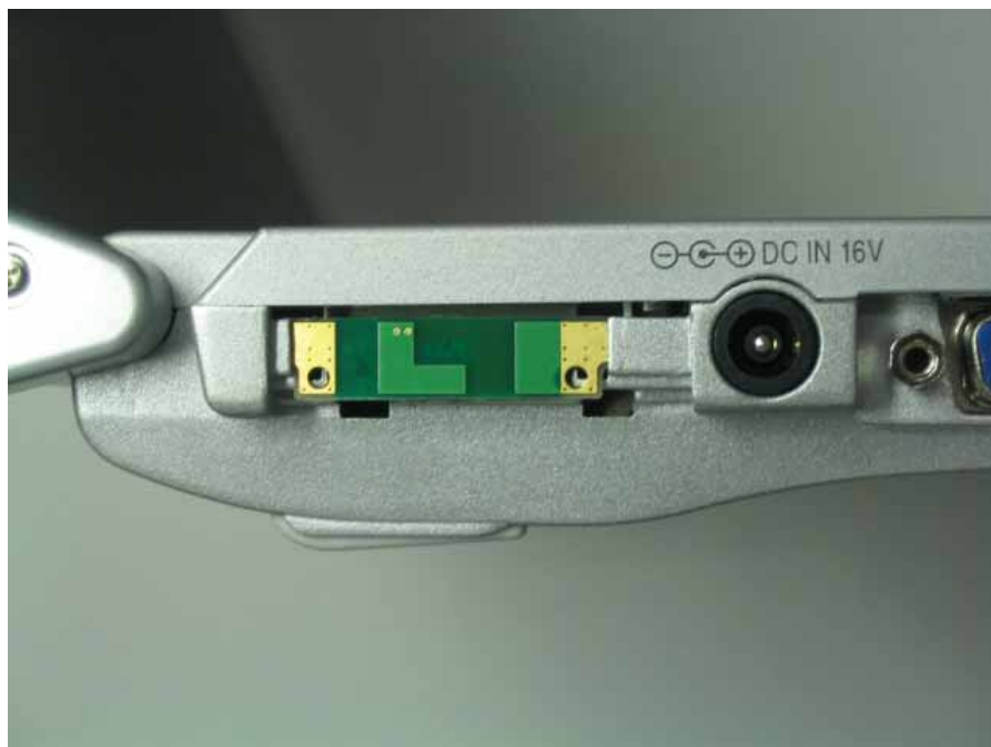
Aux TX/RX Antenna Magnified View
