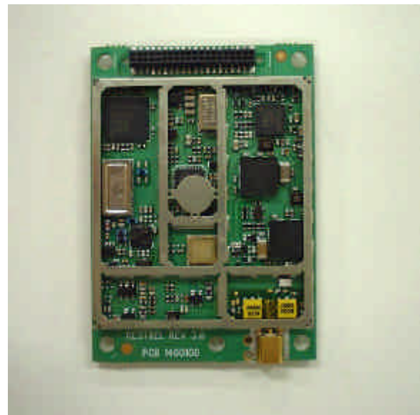
SB555 Module Interior Bottom View
