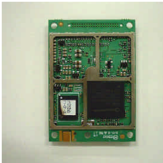
SB555 Module Interior Top View
