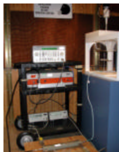
Figure A.0 Dipole Validation Test Setup
